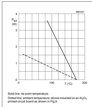
Fig.3 Maximum total power dissipation as a function of temperature.
